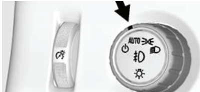
Exterior Lamp Controls here
